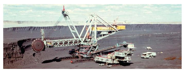
NKMZ bucket-wheel excavators have established themselves as highly reliable mining vehicles. 70% of stripping operations in the quarries of Ukraine and CIS countries are carried out by NKMZ excavators.
