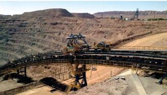
NKMZ produces conveyors of various types that are applied for opencast mining operations. These are:
